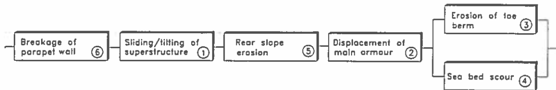
FIG. 11. Decomposition of the fault tree Fig. 8 into series and parallel systems.
